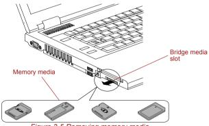
Figure 3-5 Removing memory media
